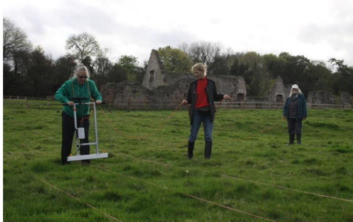
The geophys team carrying out a resistivity survey at Grace Dieu.
